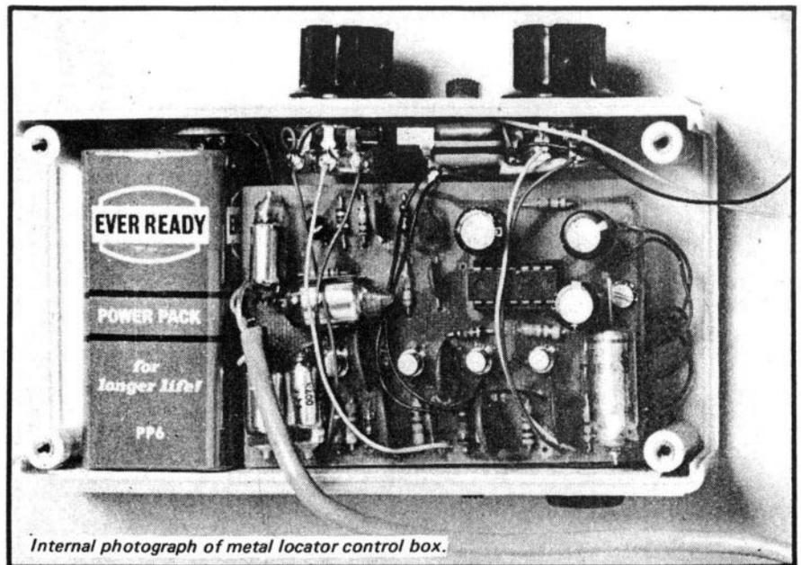
through a signal to the speaker. Bring a piece of metal near the coil and the signal should rise. If it falls in level (i.e. the crackling disappears) the coil has to be adjusted until metal brings about a rise with no initial falling. CV1 should be adjusted for maximum signal, this has to be done in conjunction with RV1.
