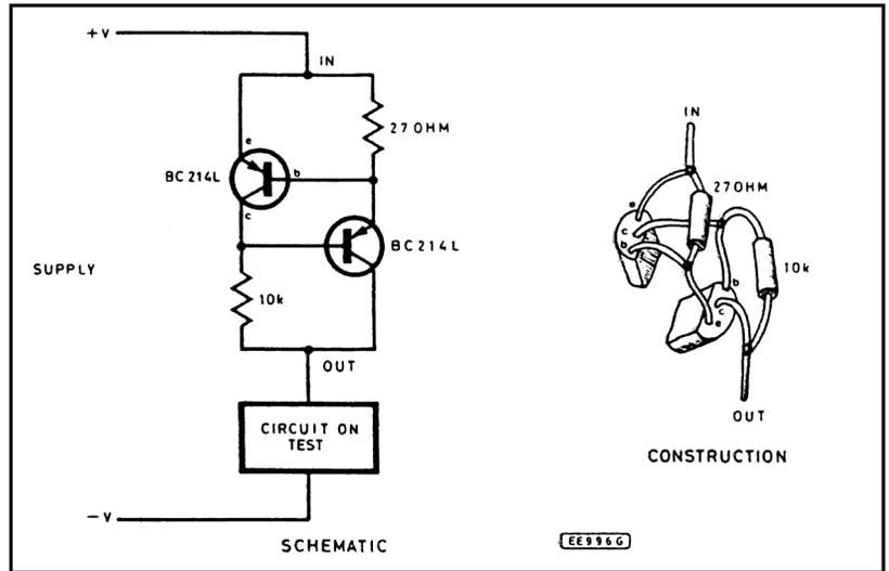
Fig. 9. Test circuit for current limiter.
