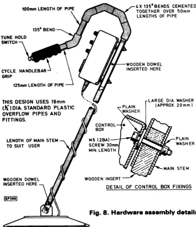
Fig. 8. Hardware assembly details
