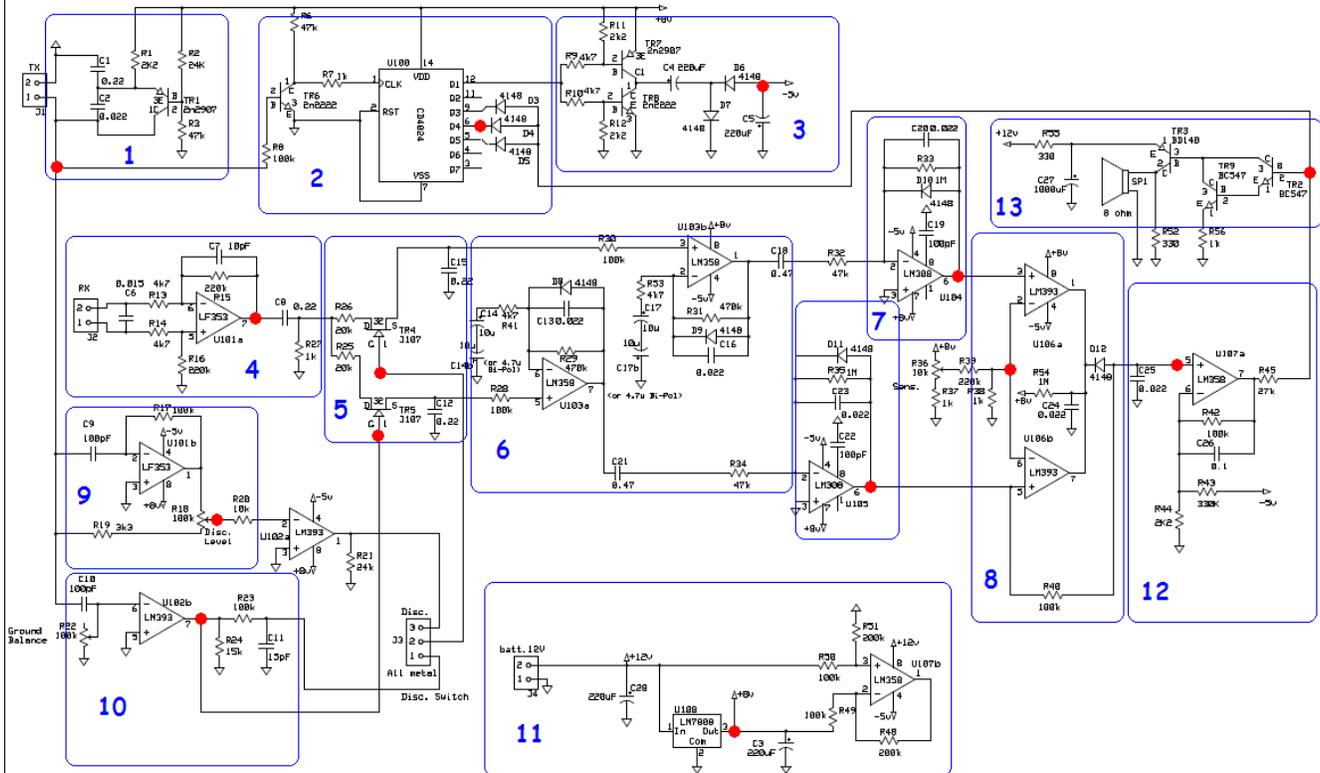
1. The basic Colpitts oscillator. Together with the transmit coil attached to J1, it provides a 14.5 kHz low power Tx signal to the coil, audio circuit, -5v converter and a signal to use as a phase comparison for the receive circuit. Tx amplitude should be in the 16V range.
