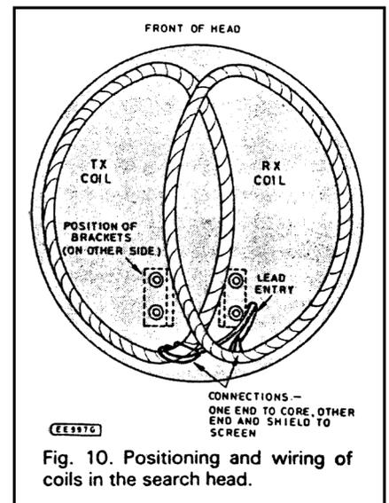
Fig. 10. Positioning and wiring of coils in the search head.
