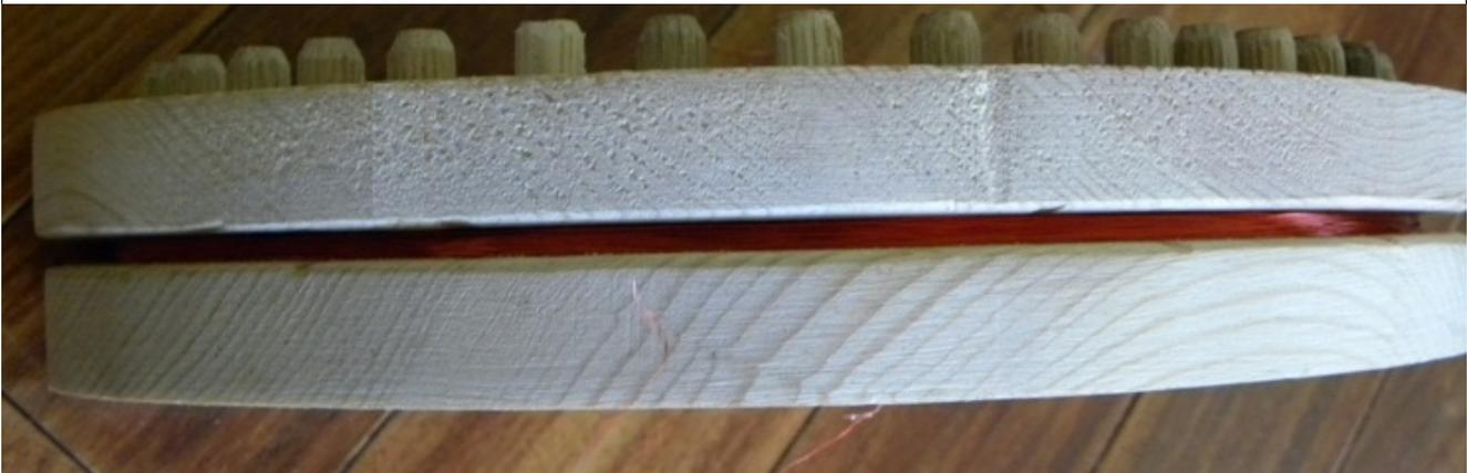
Once wire is put on a form, it's a good time to verify inductance. This can be done with an inductance meter. Or.. my favorite method is just attach the coil to your completed circuit board (J1) and measure the running frequency. The Tx should run at 14.5 kHz.
