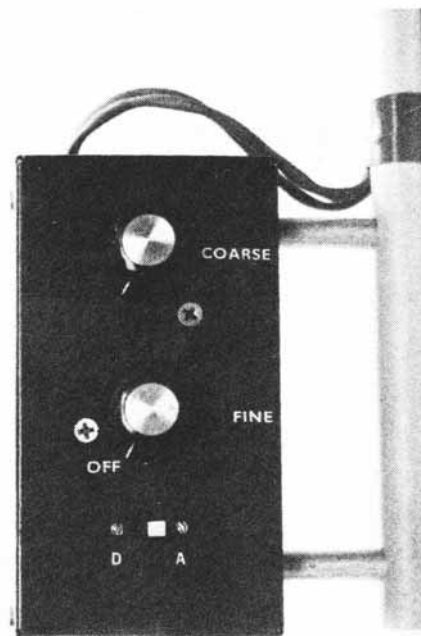
Hounddog's control head is laid out simply; there's an SPDT switch and two adjustments.
