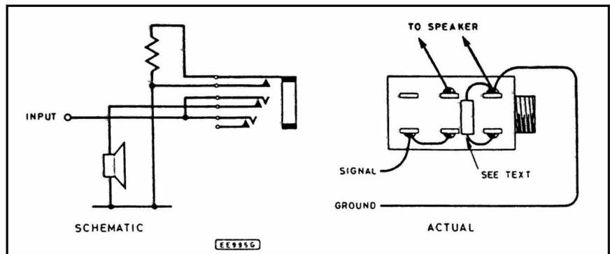
Fig. 8. Headphone socket circuit and wiring arrangement.
