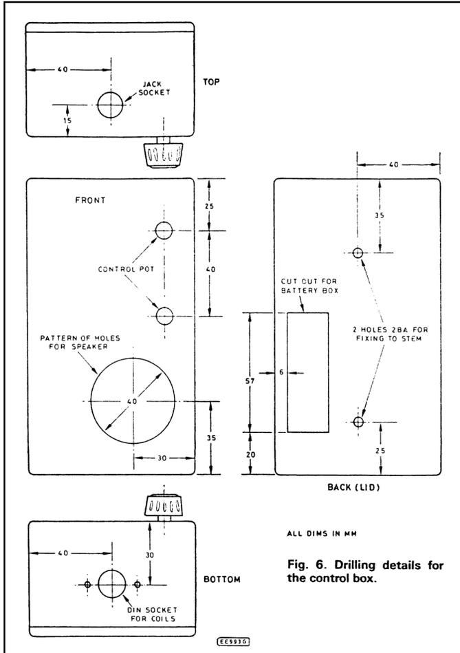
Fig. 6. Drilling details for the control box.
