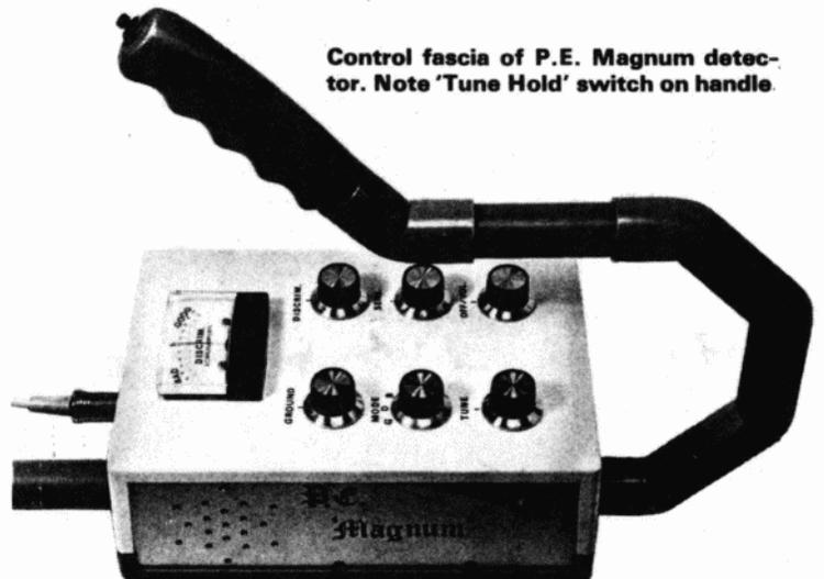
**Control fascia of P.E. Magnum detector. Note 'Tune Hold' switch on handle.**
