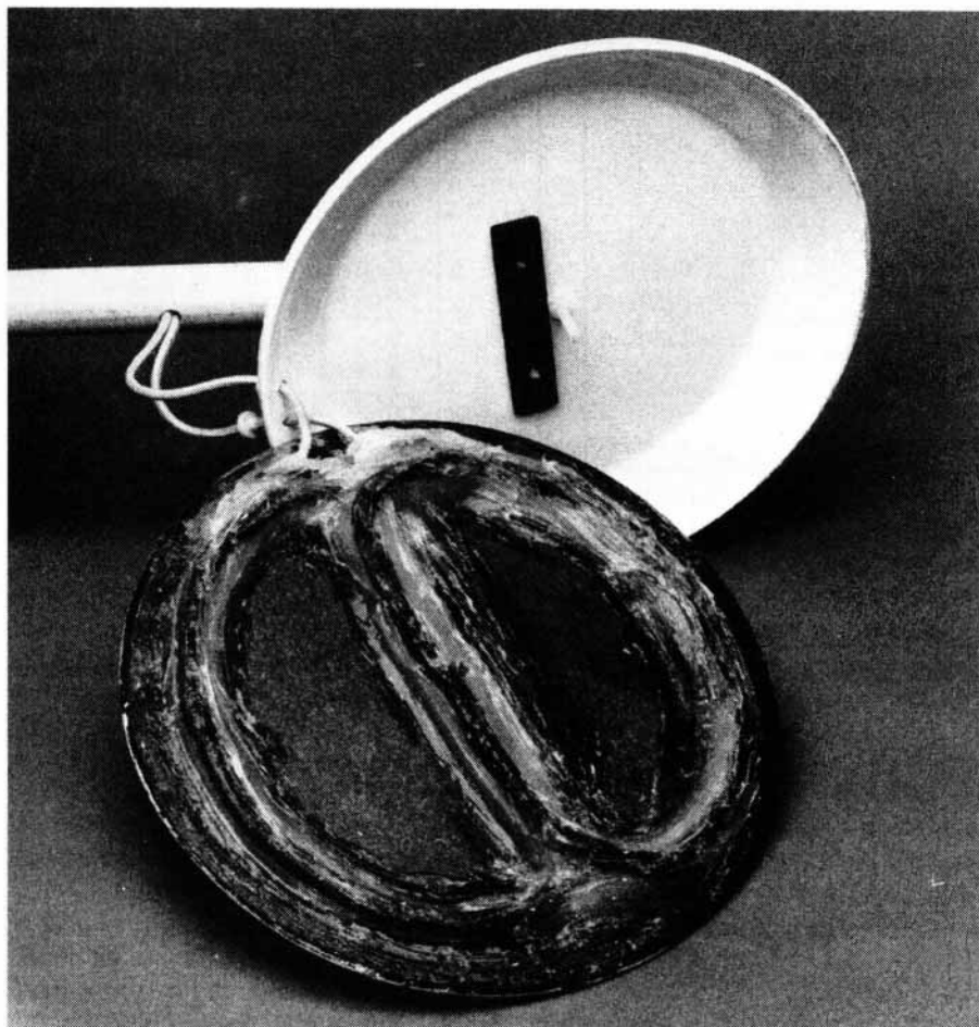
This view shows the search head assembly after the two coils have been secured to the baseboard using neutral cure silicone sealant.
