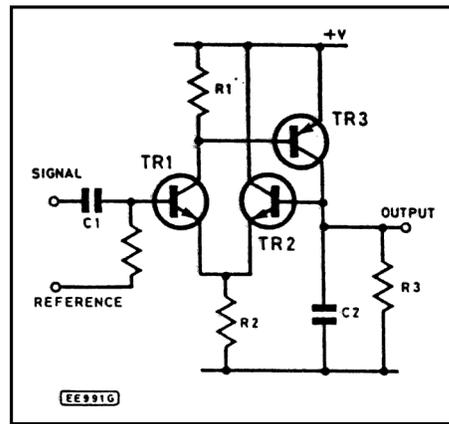
Fig. 3. The simplified peak detector circuit.
