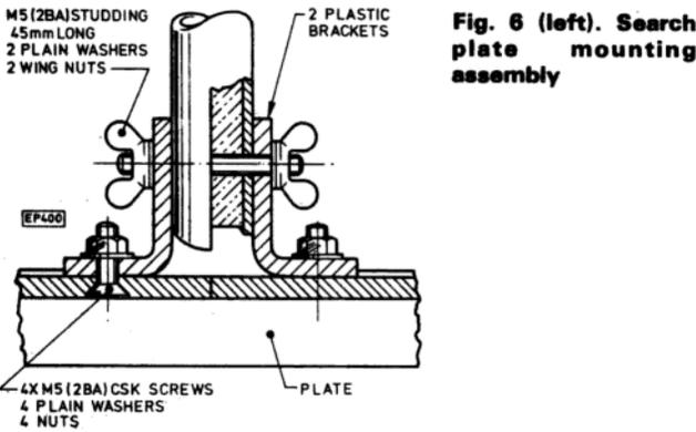
**Fig. 6 (left). Search plate mounting assembly**
