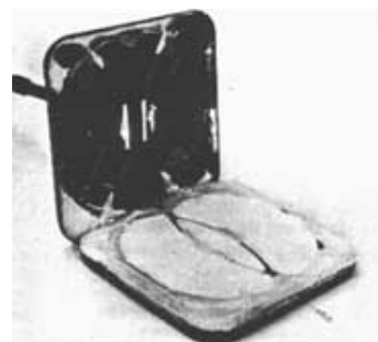
Inside the search head. The transmit and receive coils overlap by about 25mm.
