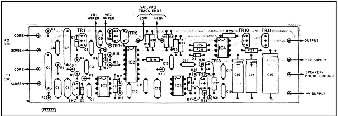
Fig. 4. Component layout on the printed circuit board.
