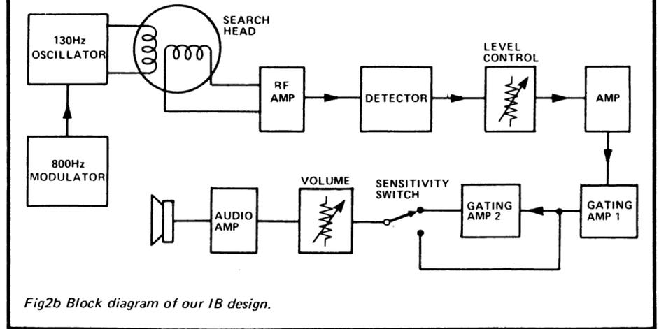
Fig.2b Block diagram of our IB design.
