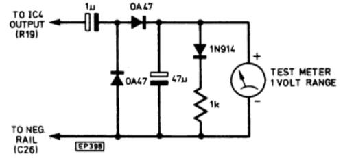
**Fig. 10. Circuit for setting up search coils**
