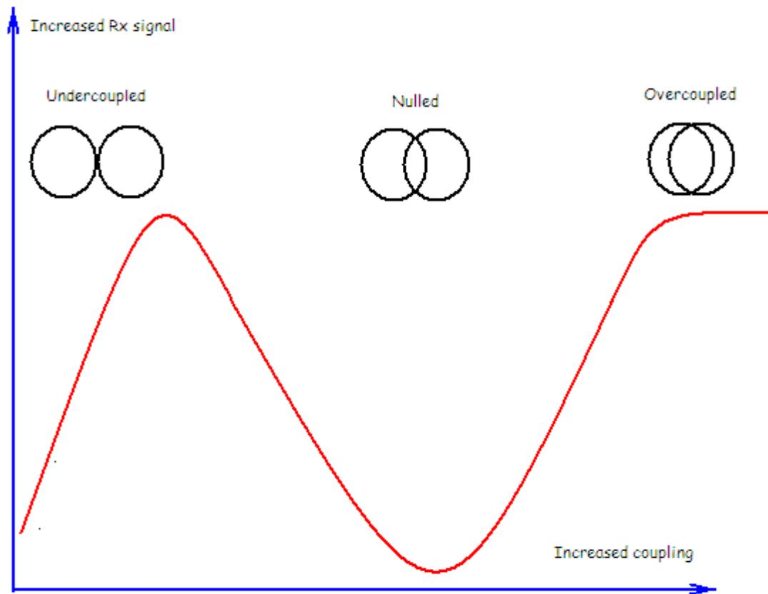
The final USB-2 cable to the circuit should be used and wires should be kept short as possible. Ideally, they should be placed inside the coil shells and the bottom coil should be secured. Power on the TGSL and adjust coil overlap while measuring the open ends of the Rx coil with a DVM in the A.C. setting. The goal is to find a sharp null in the voltage reading. You should be able to get the signal down to about 4mV but the actual reading may be subject to the frequency response of the DVM used.
