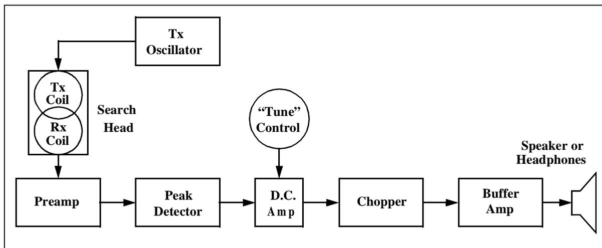
Fig. 1. Block diagram of the induction balance metal detector.
