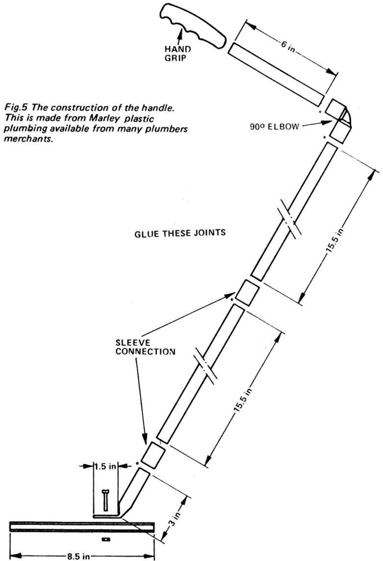
Fig.5 The construction of the handle. This is made from Marley plastic plumbing available from many plumbers merchants.
