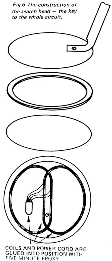
*Fig.6 The construction of the search head - the key to the whole circuit.*
