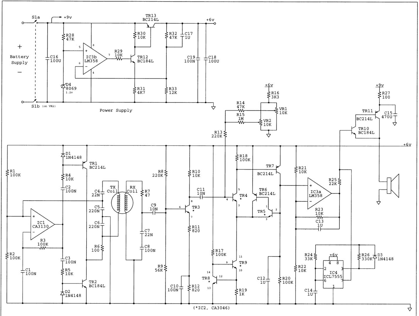
Fig. 2. Complete circuit diagram for the EE Buccaneer Metal Detector.
