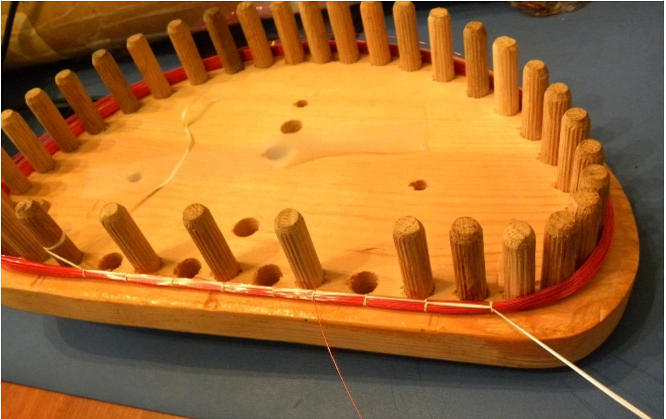
Following constraining the wires, they *must* be infused with cyan glue, so the coils become very stiff. This is very important as IB detectors are very unforgiving if not mechanically rigid!
