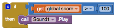
Figure 18-4. A Boolean expression used to test the value of the variable score
