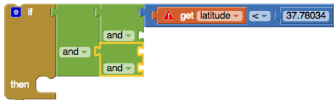
Figure 18-8. Blocks for the first test are placed into the and block
