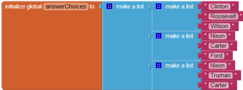
Figure 19-21. A list of lists is formed by inserting make a list blocks as items within an inner make a list block
