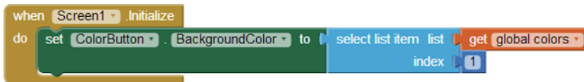
Figure 19-10. Setting the BackgroundColor of the button to the first color in the list when the app launches
