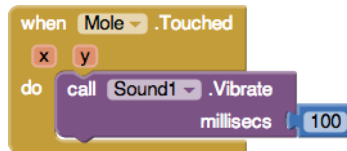
Figure 3-10. Making the device vibrate briefly (for 100 milliseconds) when the mole is touched
