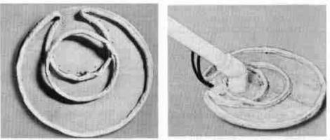
Fig. 4. The disc is shown with L1 and L2 tied in place and L3 on top.
